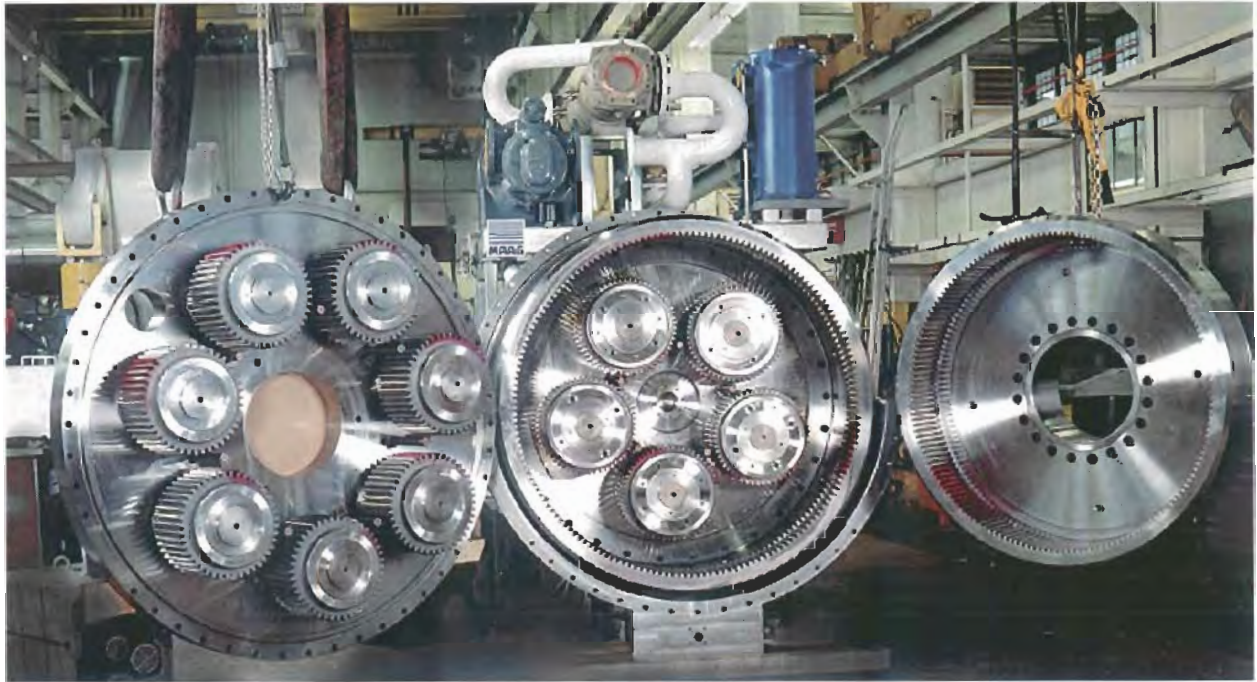
Picture1 open gearbox. Left: planet carrier II, middle: planet carrier I, right: annulus I with sun pinion II
