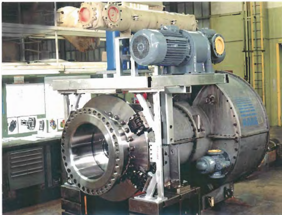
Picture1 open gearbox. Left: planet carrier II, middle: planet carrier I, right: annulus I with sun pinion II
